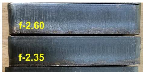
Figure 7. Photographs of 19 mm mild steel cut using Mach Ultra (Index 4) with O<sub>2</sub> assist gas. The edge quality is excellent, as with other CFX fiber lasers.
