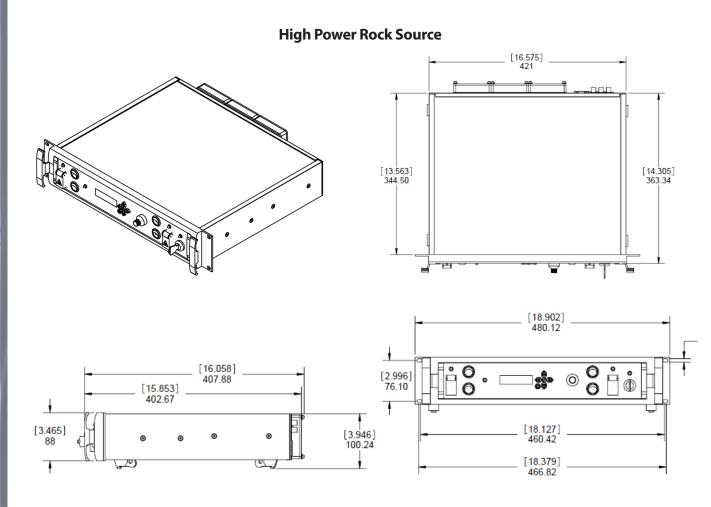
DIMENSIONS ARE IN MILLIMETERS, DIMENSIONS IN [XXX] ARE IN INCHES.
