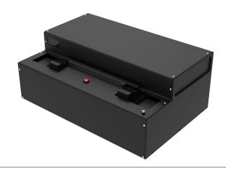
he AUTOSTRIPPER  $2^{\text{TM}}$  is designed for fast, chemical-free window stripping of optical fibers, using heated air to accomplish the often difficult task of window stripping fibers with acrylate coating diameters up to 550  $\mu$ m. The AUTOSTRIPPER  $2^{\text{TM}}$  meets the need for variable and multiple window strip lengths at high strength and ultra cleanliness.
