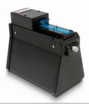
The CLEAVEMETER LIGHT<sup>™</sup> is a non-contact interferometer designed for inspecting the end-faces of cleaved or polished optical fibers with cladding diameters of 125 µm to 800 µm. It gives immediate and precise information on important end-face properties such as flatness, perpendicularity, hackles and dust. Based on the NYFORS CLEAVEMETER 3D<sup>™</sup> design, in addition to displaying sharp fringe patterns it also generates three-dimensional images of the cleaved fiber end.
