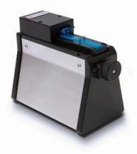
The CLEAVEMETER 2<sup>™</sup> is a non-contact interferometer designed for inspecting the end-faces of cleaved or polished optical fibers with cladding diameters of 125µm to 1200µm. It gives immediate information on important end-face properties such as flatness, perpendicularity, hackles and dust. Sampling tests as well as continuous process documentation can be carried out both easily and quickly, making this an ideal instrument for cleaver inspection and optimisation.
