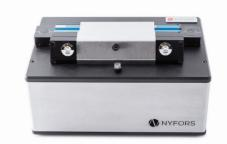
The PROOFTESTER™ is a compact and light weight instrument ideal for testing the strength of optical fibers up to 30 N. It is developed to meet all applications where a strength tests has to be performed and has a user friendly design.
