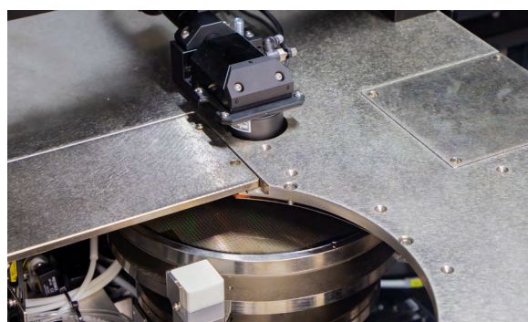
Optional upper looking chuck camera for probe-to-pad alignment
