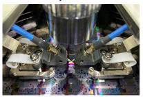
RF LTM probe arms, equipped with SmartCarrier™
