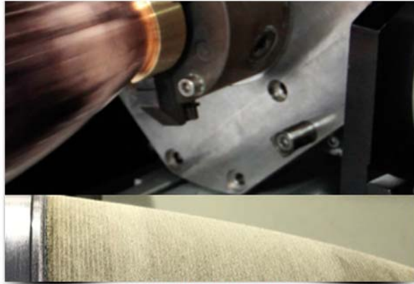
LASER CLADDING TECHNOLOGY COPPER COMPONENT + INCONEL 625 CLAD PROVIDES MECHANICAL STRENGTH TO A CONDUCTIVE COPPER PART
