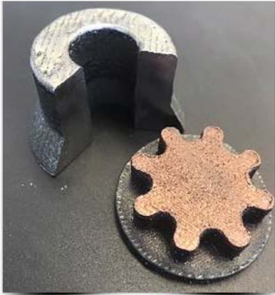
MULTI-MATERIAL COMPONENTS IN718 / IN625 / STellite 6 (LEFT) IN625 / COPPER (RIGHT)
