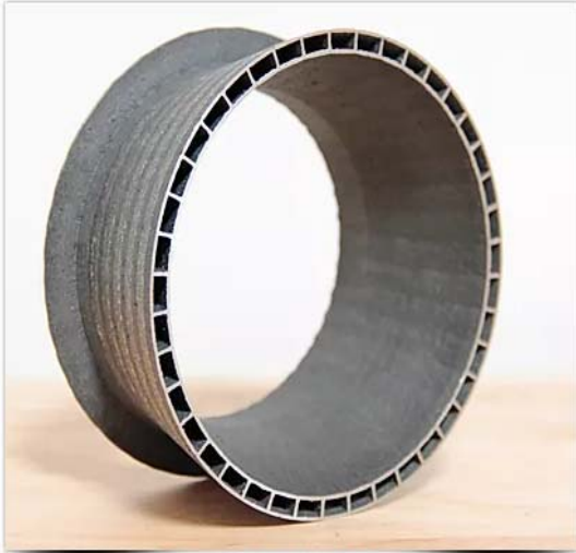
ADDITIVE MANUFACTURING TECHNOLOGY NASA ROCKET NOZZLE PART INCONEL 625
